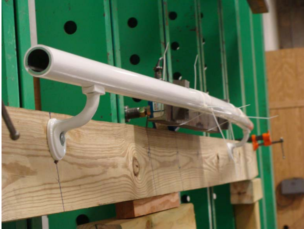
PHOTO 3: 50 plf Load Applied – Horizontal (photo taken at 300 lbf)
