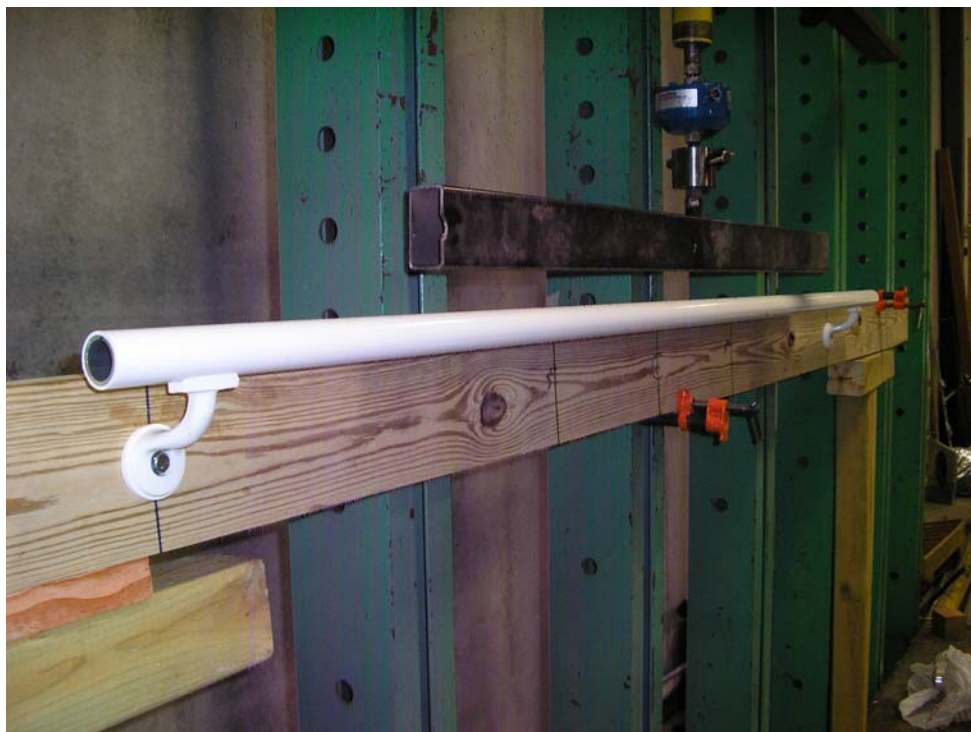
PHOTO 4: 50 plf Load – Vertical (photo of set-up, no load applied)
