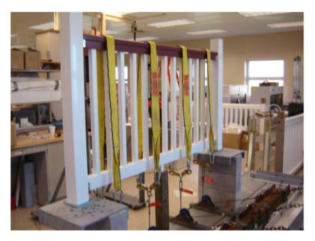
Photo No. 4 Vertical Uniform Load on Top Rail
