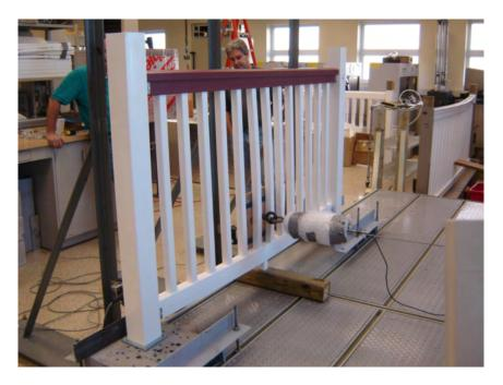
Photo No. 2 Infill Load at Bottom of Three Balusters
