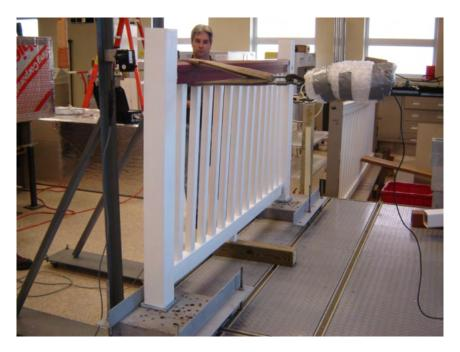
Photo No. 6 Concentrated Load at End of Top Rail (Bracket)
