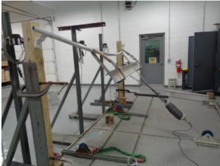
Photo No. 1 Uniform Load Test Applied at 45 degrees
