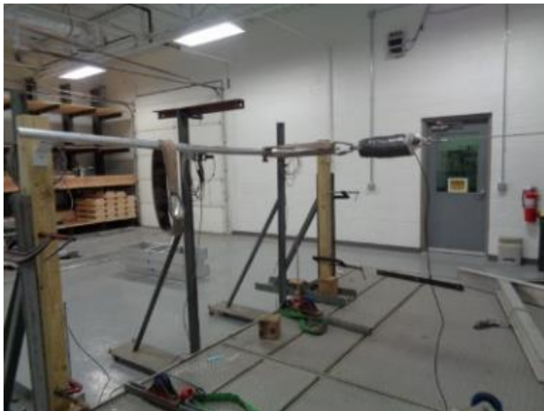
Photo No. 2 Horizontal Concentrated Load Test at Mid-Span of Handrail
